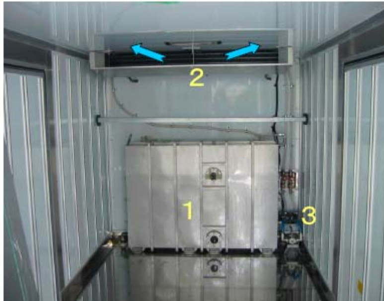
Elements of the Eco-run-cool refrigeration container: (1) dynamic ice storage tank; (2) forced convection air cooler; (3) ice slurry circulation pump (Courtesy of Professor Yukitaka Kato, Tokyo Institute of Technology, Japan). Saving up to 30% CO 2 emissions as compared to conventional on-board cooling.
