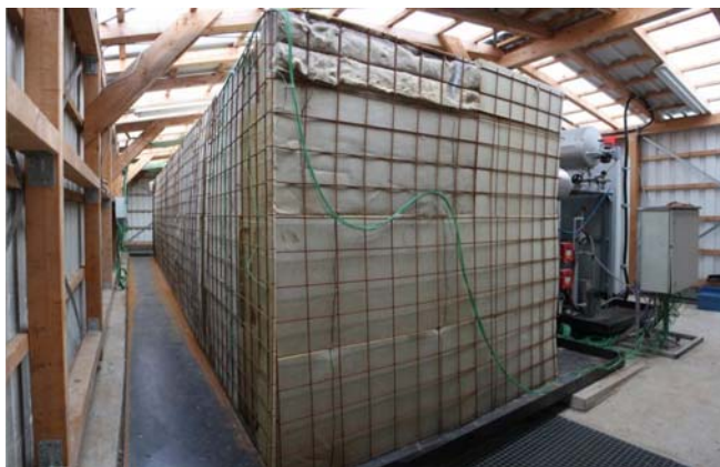
400 kWh sensible concrete storage module for heat storage in the 100-400 °C range (source DLR)
