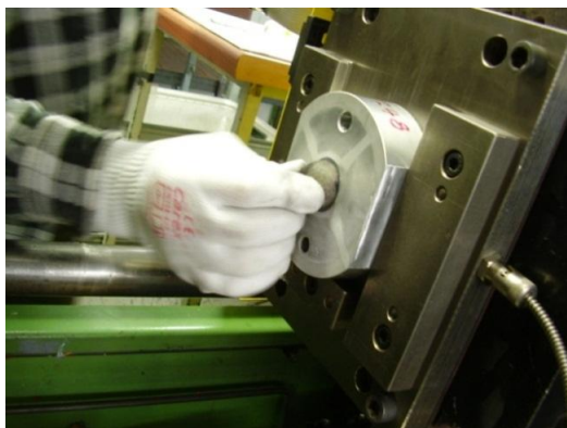
Figure 25: Encapsulation of the PCM-Blanks (left) and PCM-Balls ready for Application
