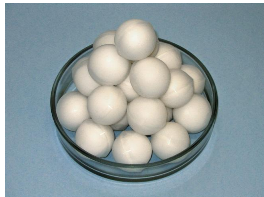
Figure 25: Encapsulation of the PCM-Blanks (left) and PCM-Balls ready for Application
