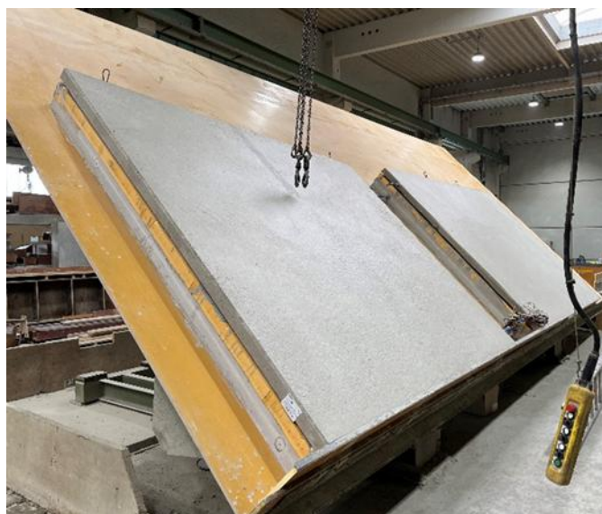
Figure 46: Production of sandwich façade elements at the precast plant Otto Knecht GmbH. Source: Karsten Rauber, IZES gGmbH
