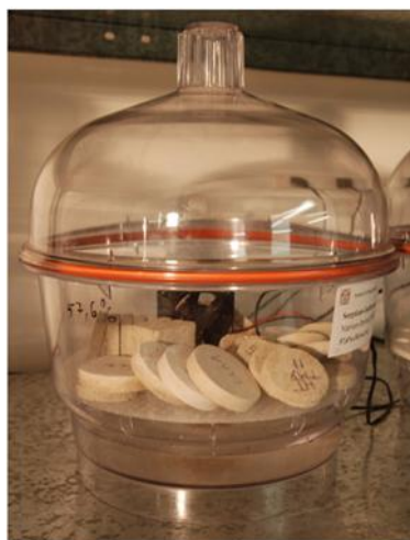
Figure 11: Desiccator with salt solution for moisture sorption measurements. Source: TU Dresden
