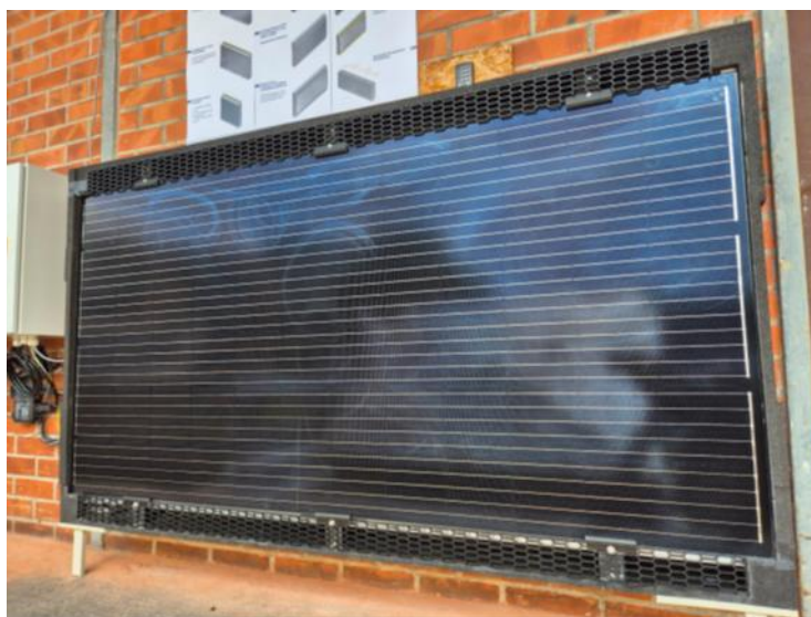
Figure 56: Functional model of the fronTherm module on the façade of Consolar's production hall in Lörrach. Source: Karlsruhe Institute of Technology, Building Science & Technology Group
