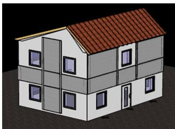
Figure 49: Renovated SFH100 using LEXU+ sandwich façade elements (dark gray) and conventional ETICS (light gray). Source: IZES gGmbH
