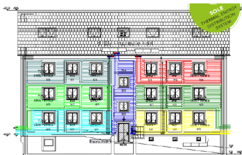
Figure 58: Schematic of CEPA zoning for TABS retrofit in a multi-family house. Individual colors represent individual hydraulic zones in the building envelope that correspond to the living units in the billing, ensuring flat wise energy supply as basis for billing. Source: Townern3000, presentation at the 35 th ES TCP On-Seminar, 16.10.2025
