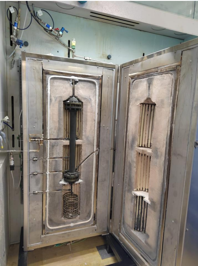
Fluidized bed reactor in Inconel up to 900 °C
