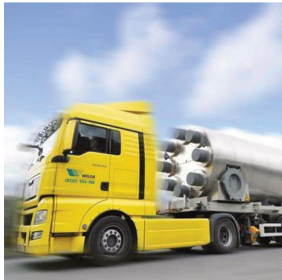
Figure 3: Mobile sorption storage for waste heat recovery in Hamm, Germany (© ZAE Bayern)
