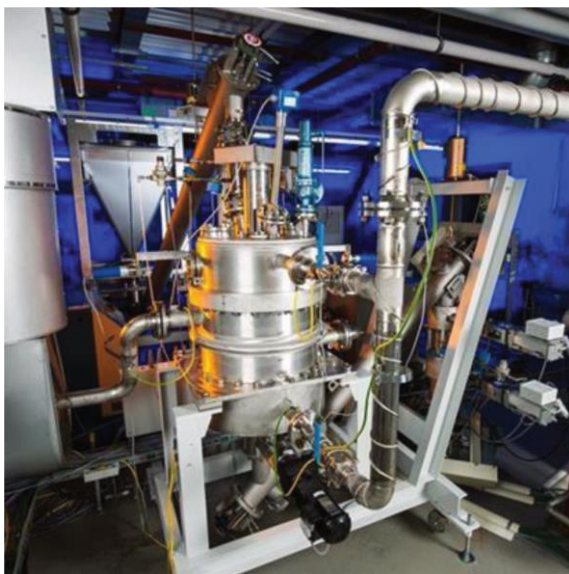
Figure 2: Laboratory installation for thermochemical high-temperature storage (10 kW/100 kWh) (t., l.), experimental setup for thermal valorisation of waste heat at temperatures > 140 °C (1 kW) (r.) (© DLR)
