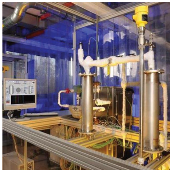
Figure 2: Laboratory installation for thermochemical high-temperature storage (10 kW/100 kWh) (t., l.), experimental setup for thermal valorisation of waste heat at temperatures > 140 °C (1 kW) (r.) (© DLR)
