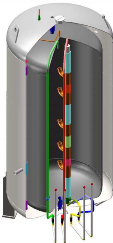
Figure 1: Bivalent sensible vacuum super-insulated-water buffer storage by manufacturer Hummelsberger (2-50 \text{m}^3 , vakuumpufferspeicher.de) with patented stratified loading system and external heat exchangers (not in picture) developed at ZAE Bayern (BMU grant # 0325964 A)
