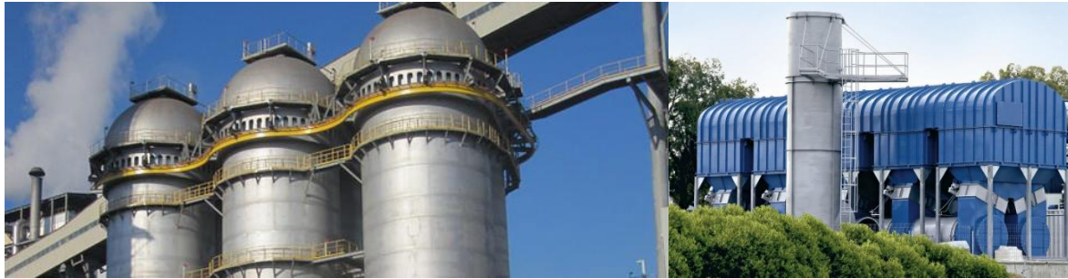
Figure 1: Cowper in a blast furnace process (left), thermal-oxidative exhaust air purification (right) (sources: [1], [2])
