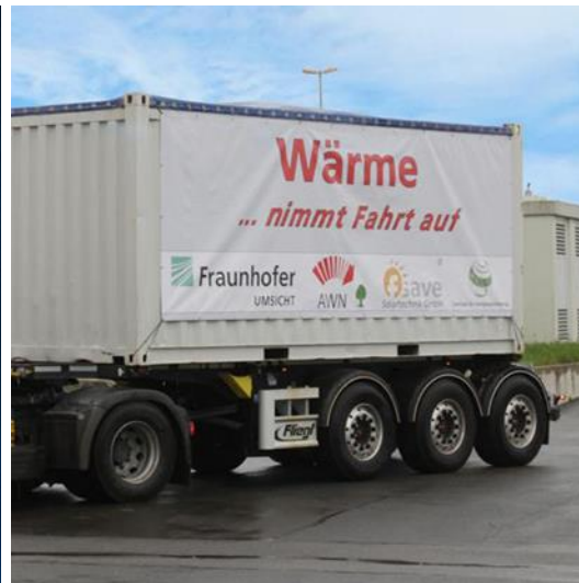
Figure 3 : Waste heat utilisation with a mobile latent heat storage used by the waste management company of the Neckar-Odenwald district
