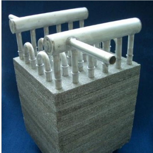
Figure 2: High-performance latent heat storage unit (without housing) with aluminium fibre structure for increased heat conduction. Laboratory model: structural volume 10 l, continuous output 2 kW, peak output 10 kW
