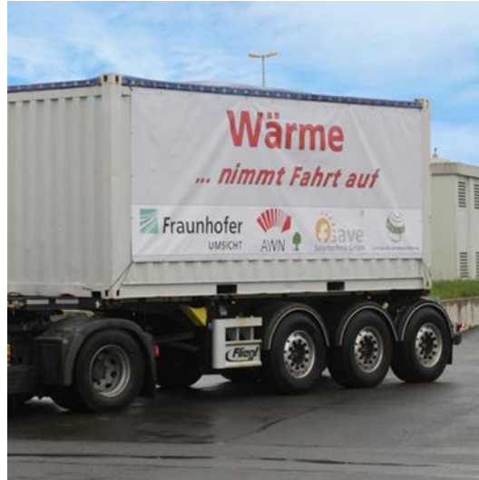
Figure 3: Waste heat utilisation with a mobile latent heat storage used by the waste management company of the Neckar-Odenwald district (© Fraunhofer UMSICHT)
