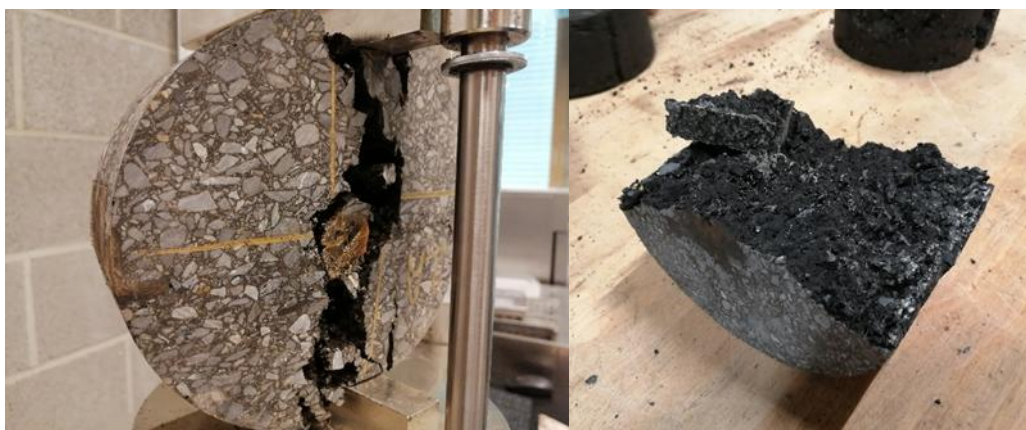
Figure 3. Post-failure resistance behavior of reference and HHP specimens in ITS test
