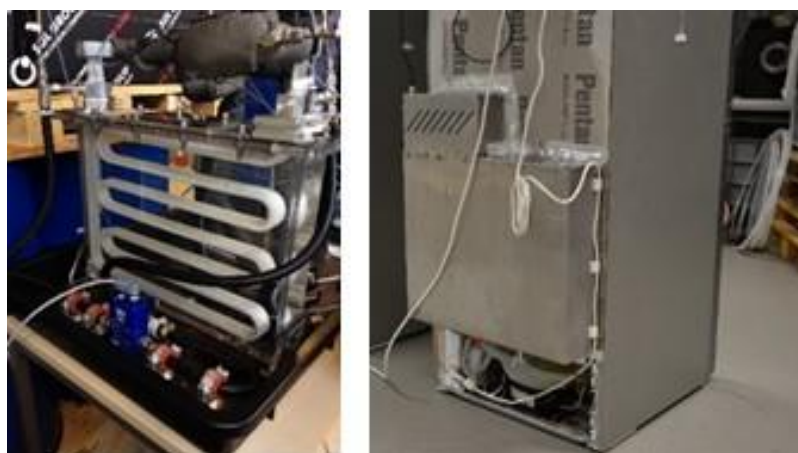
Figure 6-4: Latent cold storage within a fridge/freezer combination.
