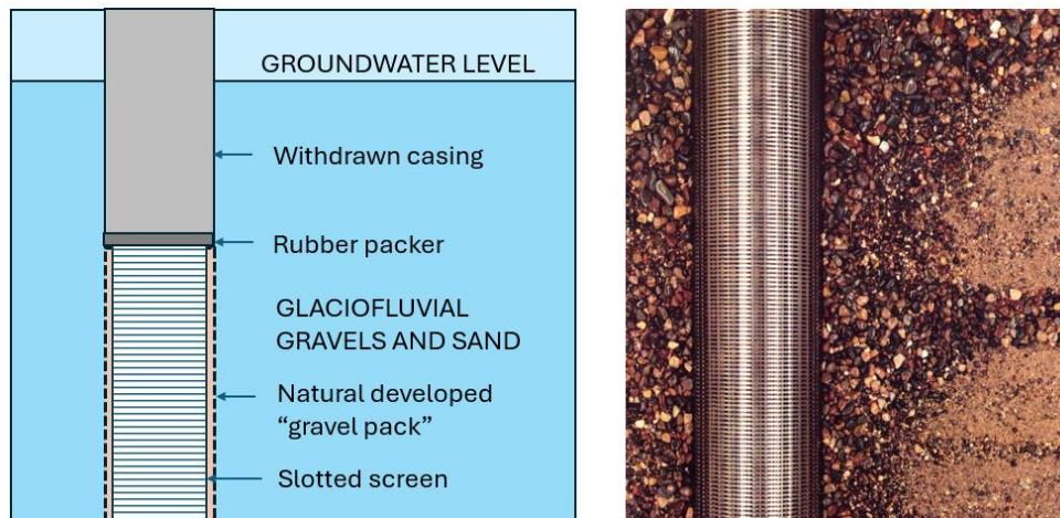
Figure 12. Natural developed gravel pack wells. Photo: From Driscoll (1986)
