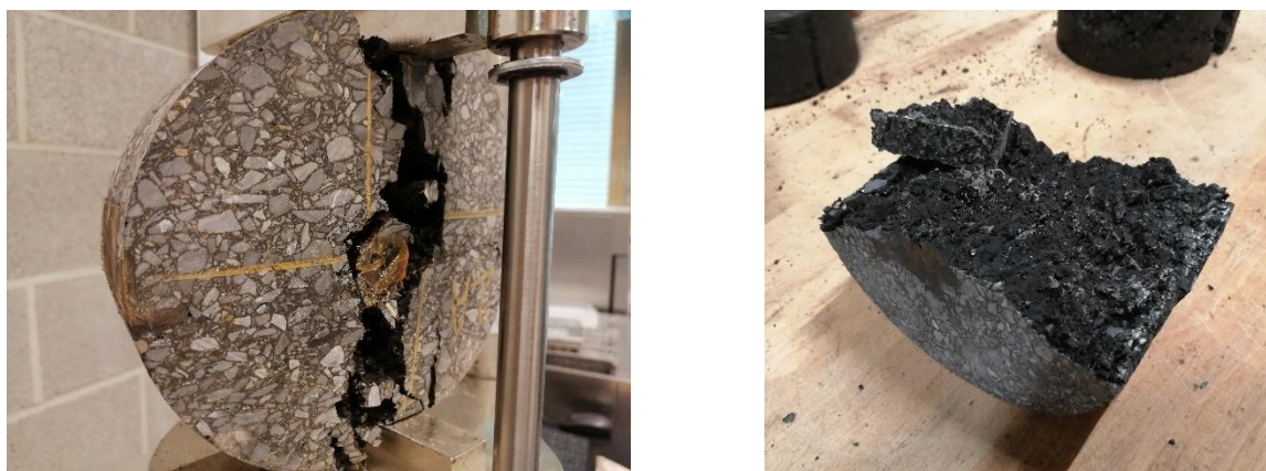
Figure 25. Post-failure resistance behaviour of reference and HHP specimens in ITS test
