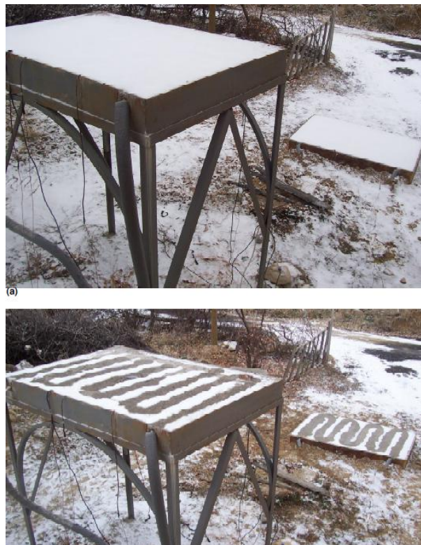
Figure 11. Initial (first picture) and intermediate (second picture) snow melting process on slabs. (from Balbay & Esen, 2010)
