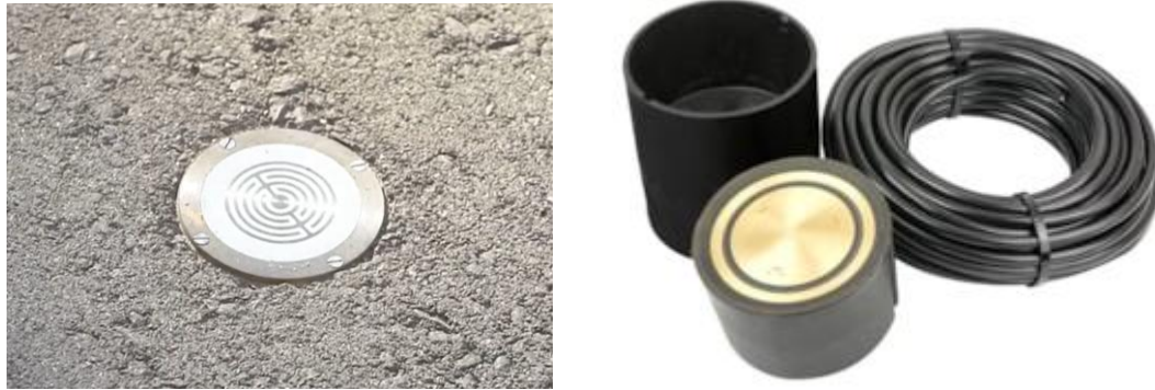
Figure 9 Embedded sensor in a concrete pavement.
