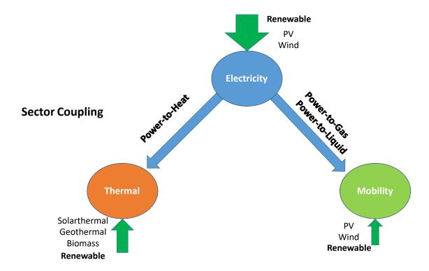
The figure above shows the coupling of the three sectors electricity, thermal (heating and cooling) and mobility, which can be realized by different technologies like power-to-gas or power-to-heat. Each sector can have its own direct renewable input. However most of the expected input will come from the electricity sector.
