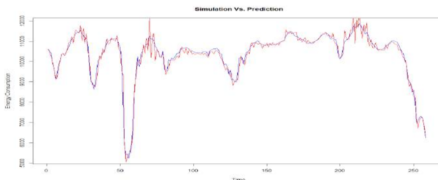
Figure : Predicted heating demand schedule vs. simulated demand profile of community 1; Last 11 Days of December
