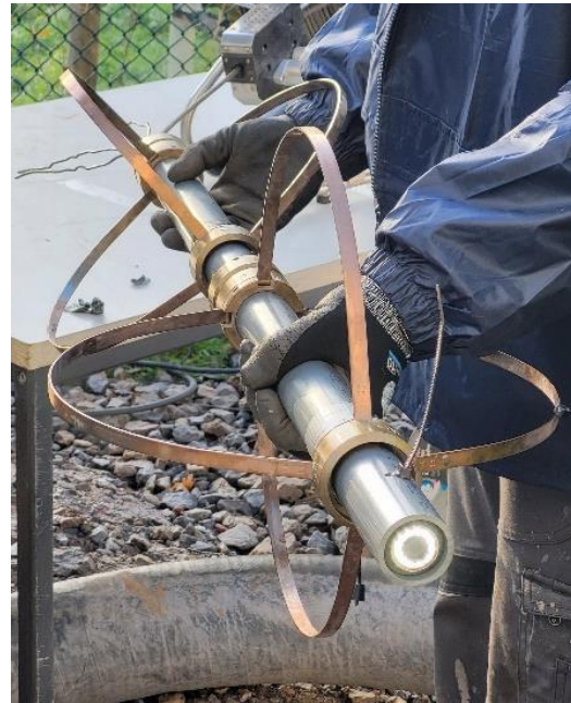
borehole camera with centralizers
